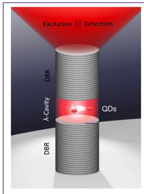
Figure 1: The semiconductor microcavity including the light coupling from the top facet. The sample, shaped into a 2 micron diameter pillar, consists of two GaAs/Aluminium Gallium Arsenide DBR's (Distributed Bragg Reflectors), and a one wavelength thickness GaAs spacer (the cavity) hosting a layer of Indium Gallium Arsenide quantum dots (QDs).
